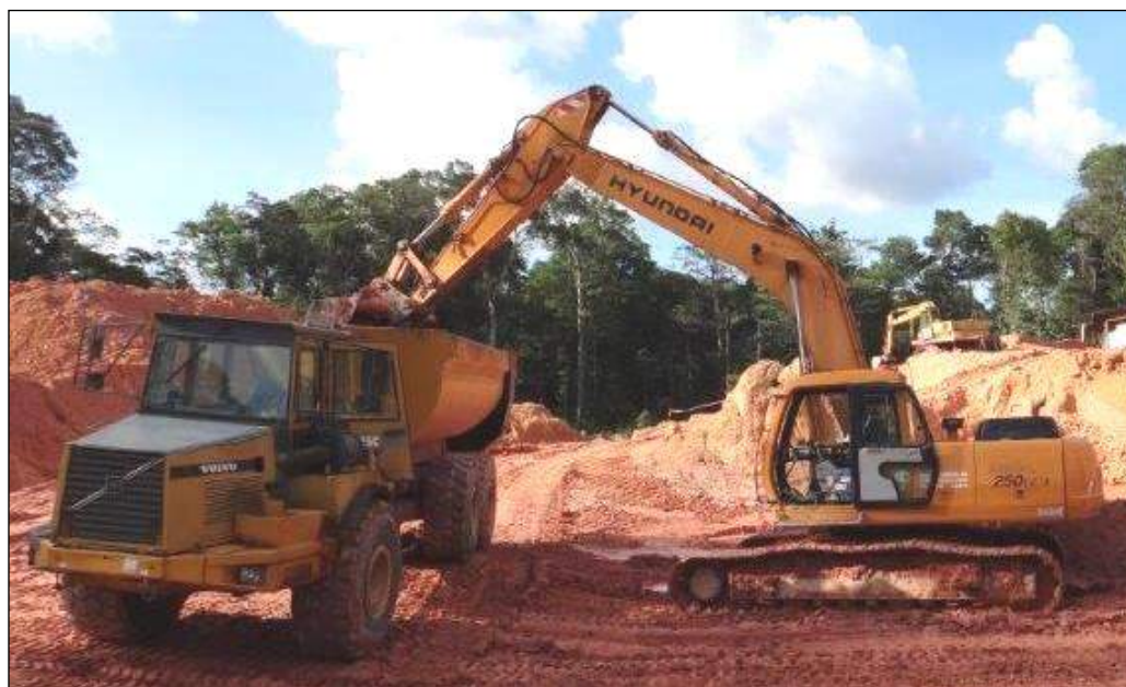
Figure 14 : Pelle HYUNDAI 250 LC3 chargeant Dumper VOLVO A25C
