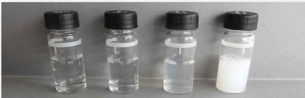
FIGURE 9 : ETALONS DU TURBIDIMETRE HI 98712 (0/15/100/750 NFU)
